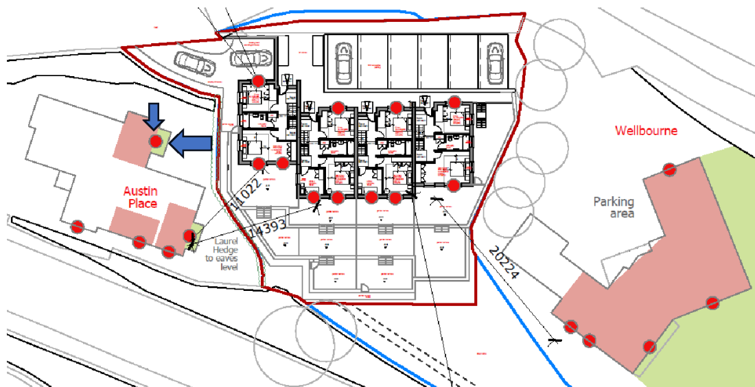
Figure 2: Arrows have been added to this plan extract to indicate living room windows at the closest apartments at Austin Place. Distances to other adjacent habitable room windows are indicated on the plan (measurements in millimetres; for example 11022 = 11.02m).
